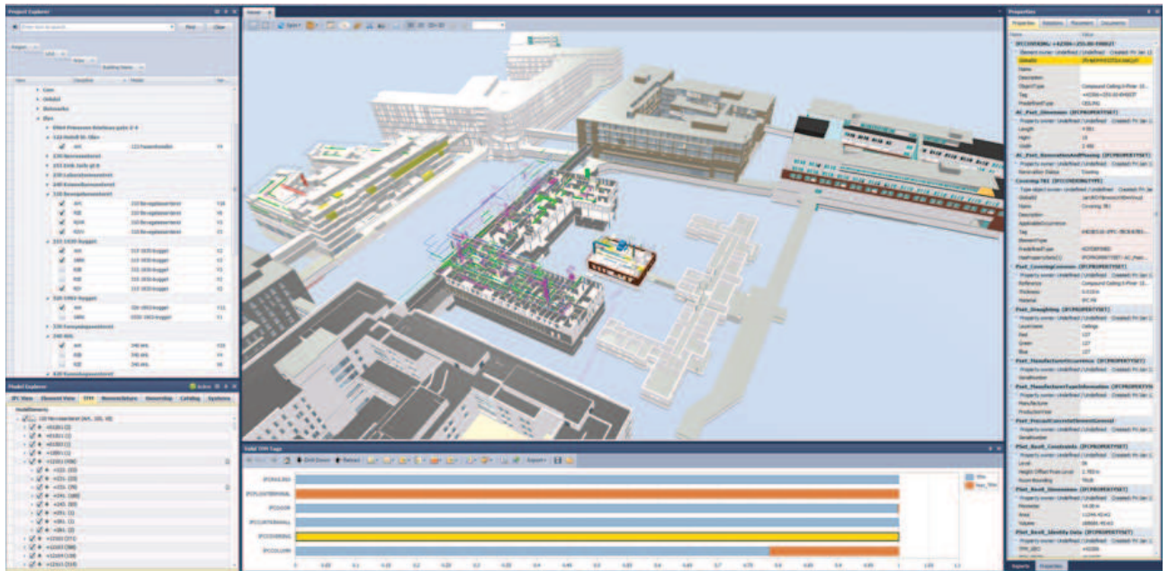
Fig 5: The model server consists of a collection of integrated BIM models with property sets, documents, methods for evaluating and checking the models and other turn key functions.
