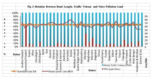
Fig. 3: Relation between road length, traffic volume and noise pollution load.
