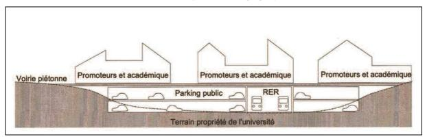
Ill. 12. The functioning of the slab. The diagram shows how the ground below – essential for long-term connectivity - remains the property of the university while the infrastructure and buildings are leased (for up to 99 years) to public and private investors.
