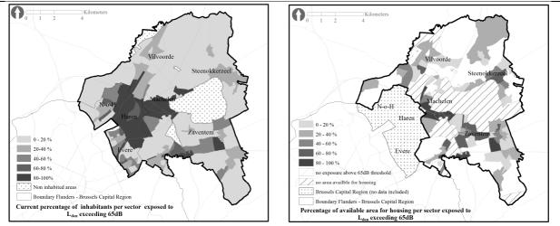
Figure6: Currentand potential exposure to Lden > 65dB (source: own map based on noise maps issued by LNE 2013 and BIM 2006)
