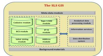
Topo 500 module – Topographic information in scale 1:500 module BCS module – Building cadastral surveing module ET IS module – Encumbred Territories IS module Fig.4: SLS GIS structure. [17]
