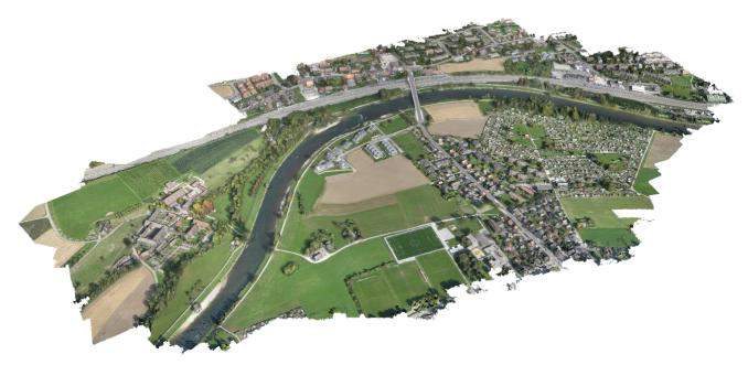
Figure 4: Processed high resolution digital surface model (DSM) with orthophoto texture of an Unmanned Aerial Vehicle (UAV). The data shows a part of the case study area of Schlieren (Canton Zurich, Switzerland) and has an accuracy of 8 centimeters (DSM and orthophoto).
