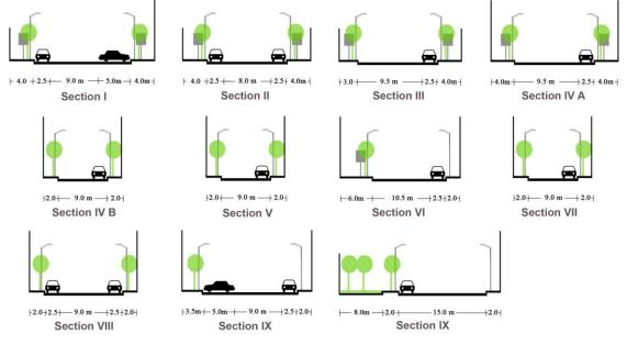
Figure 10: Detailed Street Profiles at the Different 10 Sections
