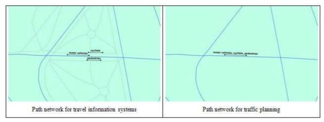
Fig. 2: Different granularities / reduced networks / transformation of traffic modes
