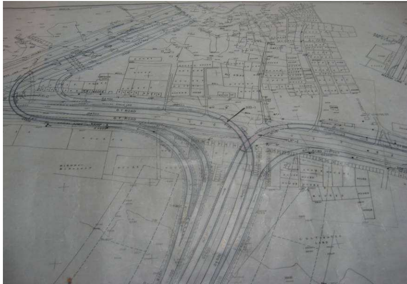
Figure 4 Right of Way of proposed Ring Road II overlaid on Survey Plan
