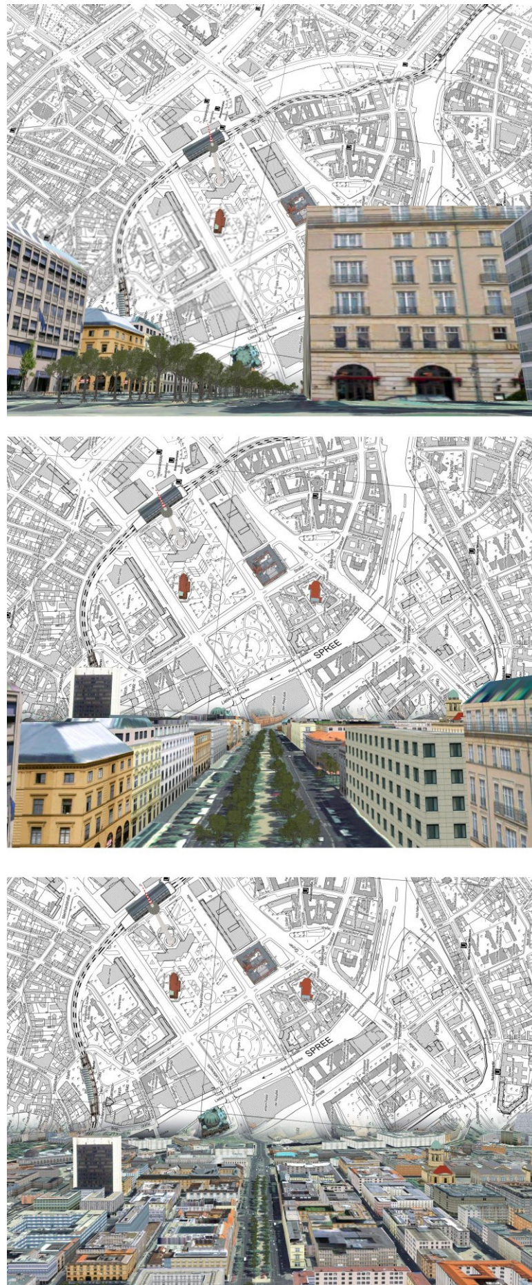
Fig. 6: Degressive perspective view at various camera heights. Produced by the LandXplorer system, based on Lorenz et al 2008.
