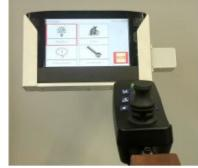
Fig. 2: The MOVEMENT modular prototype consists of a semi-autonomous robotic platform able to dock to various application modules like chairs, tables, ICT terminals and thus can provide mobility of persons, objects and information (left: robotic mobility platform moving a chair, middle: platform fetching a table with ICT terminal, right: touch screen and joystick for assisted driving mode.
