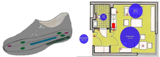
Fig. 4: Research projects in the Living Lab Schwechat: eShoe (left) a wearable embedded system for fall prevention and recognition, eHome (right) a wireless sensor network for assisted living of older persons including support in case of an emergency.
