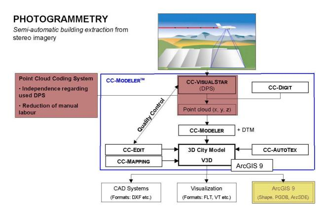
Figure 1: Workflow for Updating of 3D-city models in CyberCity processes and the management with ESRI Arc products
