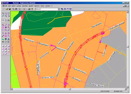
Figure 12: Transport network derived from commercial European digital data source including one-ways (red links) and turning prohibitions (violet links)
