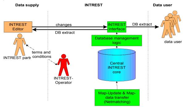
Figure 15: Principle workflow of INTREST
