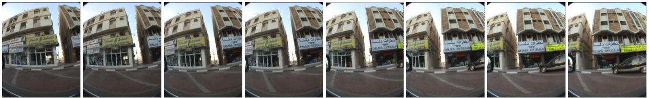
Figure 5: De-compiling the video stream into thousands of still images taken from slightly different locations on the vehicle trajectory.
